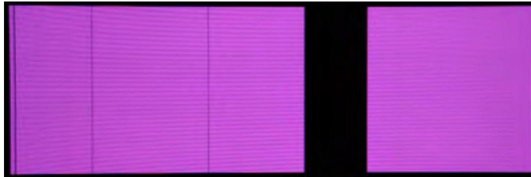
IGNIS full solution (TFT and OLED burn-in are compensated)
