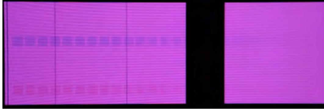
IGNIS OLED burn-in solution is off (TFT is compensated)
